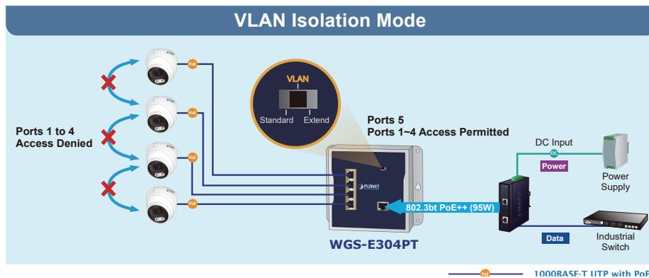
In the "Extend" operation mode, the WGS-E304PT operates on a per-port basis at 10Mbps duplex operation but can transmit data over a distance of up to 250 meters overcoming the 100m limit on Ethernet UTP cable. With this brand-new feature, the WGS-E304PT provides an additional solution for distance extension, thus saving the cost of Ethernet cable installation.
